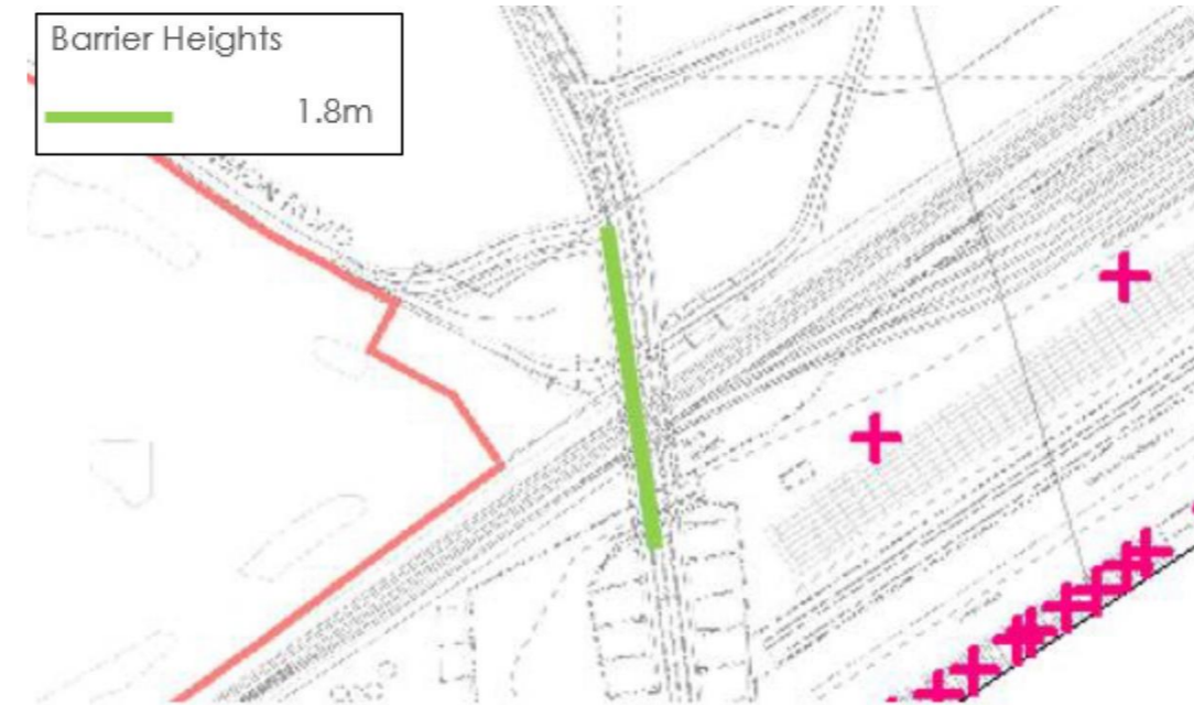
Fig 44. Noise Barrier on new Bridge on A47 Link Road
