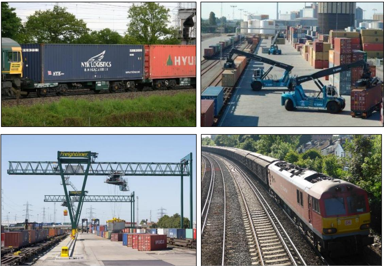
Figure 1 Examples of likely operations at an SRFI. Top left - intermodal wagons and containers. Top right - intermodal handling using reach stackers. Bottom left - intermodal handling using rail mounted gantry cranes. Bottom right - a train of conventional wagons
