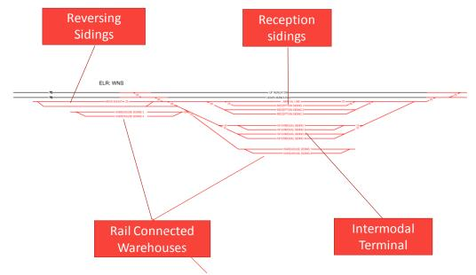
Figure 6: Conceptual Rail Layout Showing Key Features
