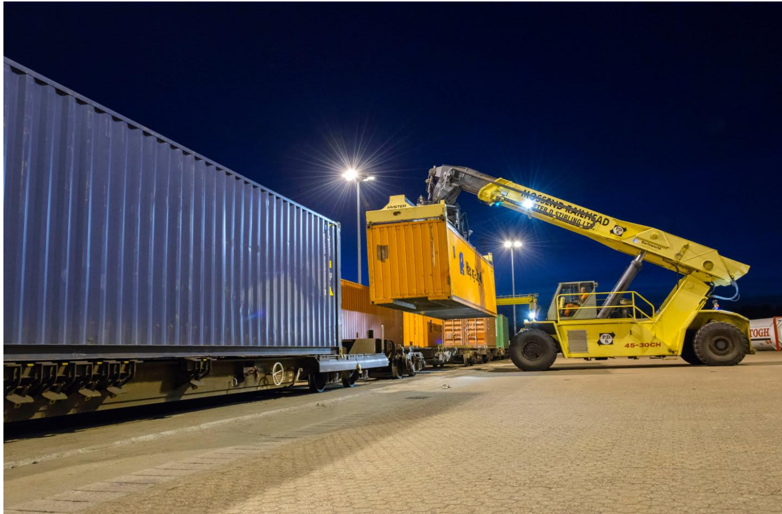
Figure 5-1 - Reachstacker operating in a railport
